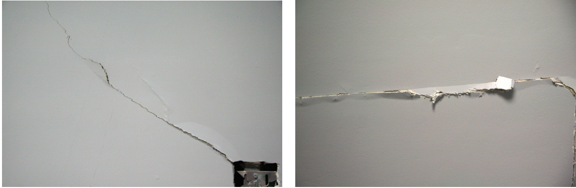
Figure 9: Examples of damage stage 2 (tests by R. Retamales et al. 2007, photos by E. Miranda).
